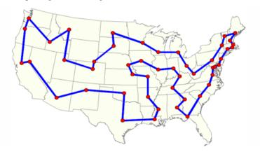
Formally, the graph is described by G = (V, A), where V is the collection of N vertices,  $A = \{(i, j) : i, j \in V\}$  is the set of edges with cost  $c : A - > \mathbb{R}$ ,  $c : (i, j) - > c_{i, j}$ , where  $c_{ij}$  is the distance from node i to node j. Lastly,  $x_{ij}$  are boolean variables such that  $x_{ij} = 1$  if the edge (i, j) is active. One formulation of the problem is (known as the "cutset" formulation):
